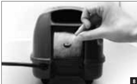
3. Replace the filter media into the filter cavity.
